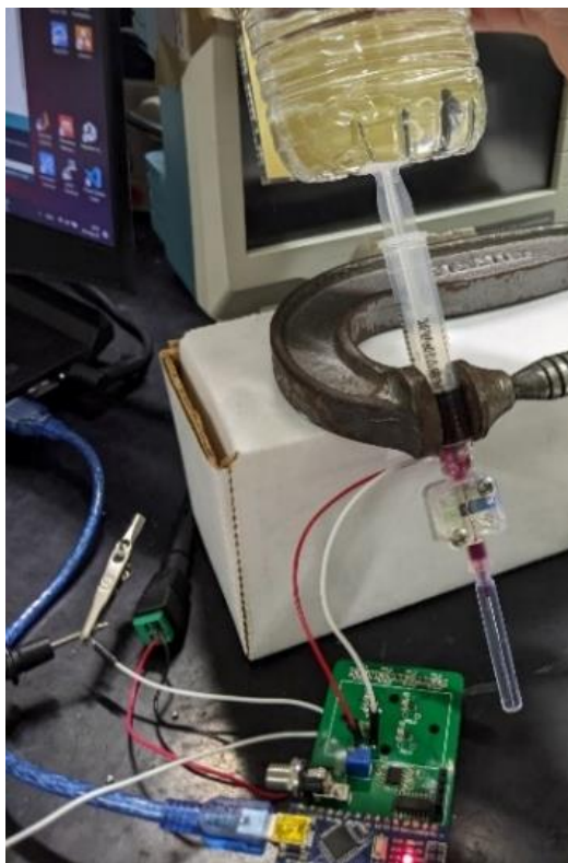
Figure 13 The experiment setup. The water bottle is about to be released on the syringe plunger. The PCB is connected to the valve unit via 2 wires, red and white and connected to the computer via the blue USB cable
